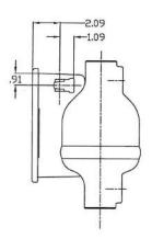
Note: All dimensions in inches; all dimensions are applicable for 1.00" NPT, socket weld and butt weld.
